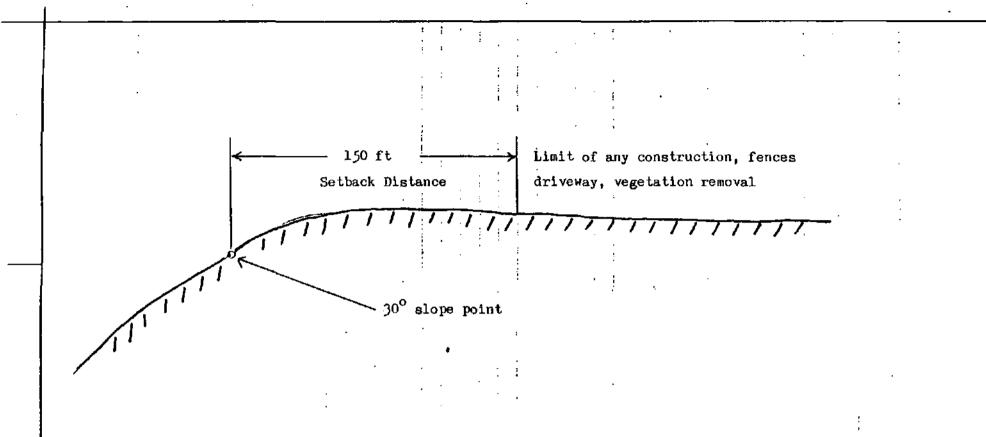
FIGURE 2. Mitigation concept to be used on lots 11 - 19, 38 - 45, and 54 - 56. As discussed in the text, insufficient space may exist on some of the lots for this concept to be executed. Field measurements are necessary to determine the precise location of the 30° point on each lot which would determine the 150 foot setback distance.
